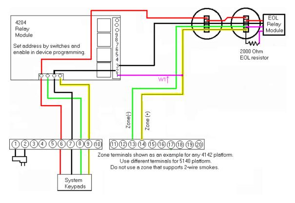
**Programming:** program zone 3 (or any zone that cannot be used for 2-wire smokes)) as normal for FIRE. Program relay#1 for smoke reset: close/stay closed. Start ZT54, stop ZT57. Set 1\*75 = 008 seconds.
